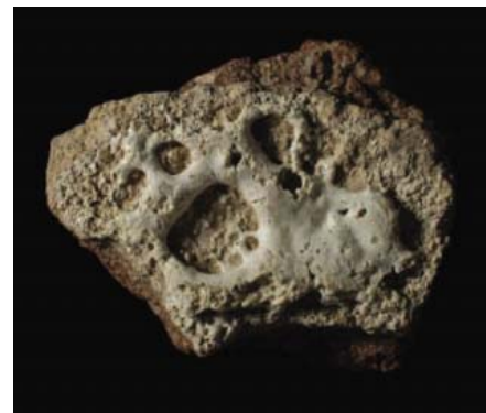
Fig. 5. Find 02/0339.0022: jar fragment with semi-reacted raw glass. The width of the object is ~4 cm. Note the residual quartz grains trapped in the fused glass and the limited wetting of the underlying parting layer by the glass.
